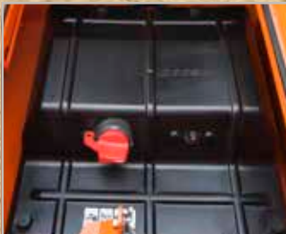
Battery cut-off switch
